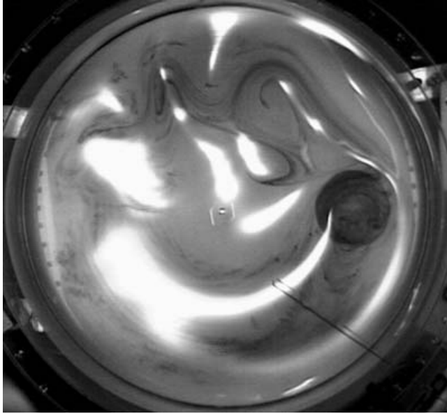
FIGURE 15. By adding background lighting, dye patterns can be viewed with altimetric images. The Rossby-wave wake downstream of the mountain is seen both in the pressure and dye fields, as is the rapid upstream penetration of the blocking region. Here dye enters upstream of the mountain from a traversing arm (thin black line) that moves back and forth along a radius. The cyclonic mean flow was suddenly initiated at time t=0 , and the image is at t=140 s. \Omega = 2.2 \text{ s}^{-1} , initial U = 7 \times 10^{-3} \text{ m s}^{-1} at r=0.4 m; blocking parameter \beta d^2/U = 3.1 .
